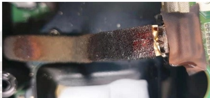
FFC cable melted
