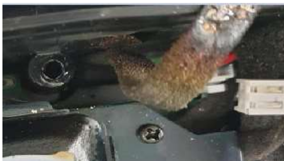
FFC cable melted
