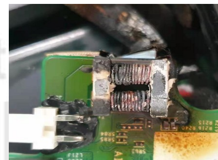
T1 component (choke) burned
